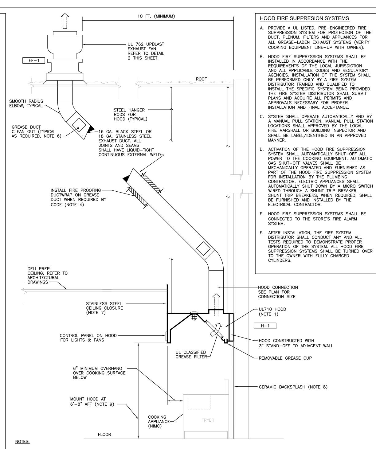
1. DETAIL SHOWN FOR GENERAL ARRANGEMENT ONLY. HOOD EXHAUST SYSTEM SHALL BE INSTALLED IN ACCORDANCE WITH NFPA 96, AND ALL STATE AND LOCAL CODES. REFER TO MANUFACTURER'S DRAWING, THIS SHEET.
